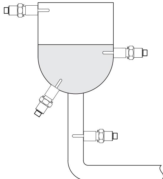
The sensor can be mounted on any point in the vessel or pipe.
