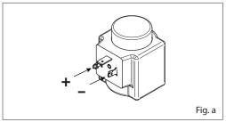
When - (minus) is supplied to the right terminal pin and + (plus) to the left (see fig. a), the valve plate is pressed down against the pilot orifice (4) by the armature spring (2).
