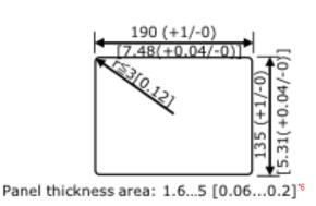
\*6 Even if the installation wall thickness is within the recommended range for the "Panel Cut Dimensions", depending on wall's material, size, and installation location of this product and other devices, the installation wall could warp. To prevent warping, the installation surface may need to be strengthened.
