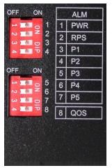
Figure 8: DIP Switches
